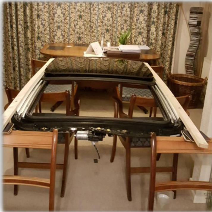
Figure 4: Testing all four corners of the roof for leakage before re-fitting
