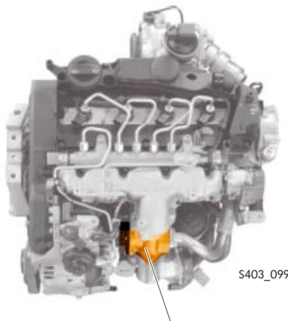
Exhaust gas recirculation valve N18 with exhaust gas recirculation potentiometer G212
