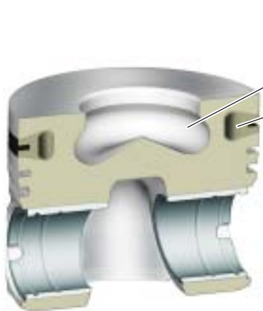
Piston from 2.0l unit injector engine
