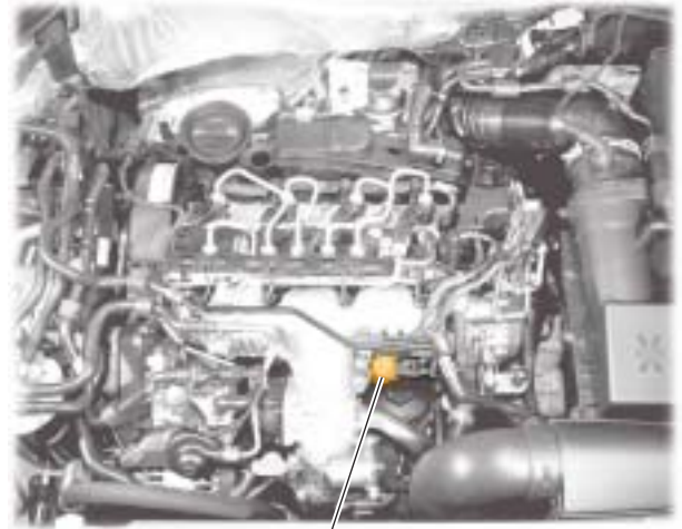
Exhaust gas recirculation cooler change-over valve N345
